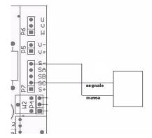
To get a signal proportional to motor speed: use one Hall sensor channel and Hall GND.
